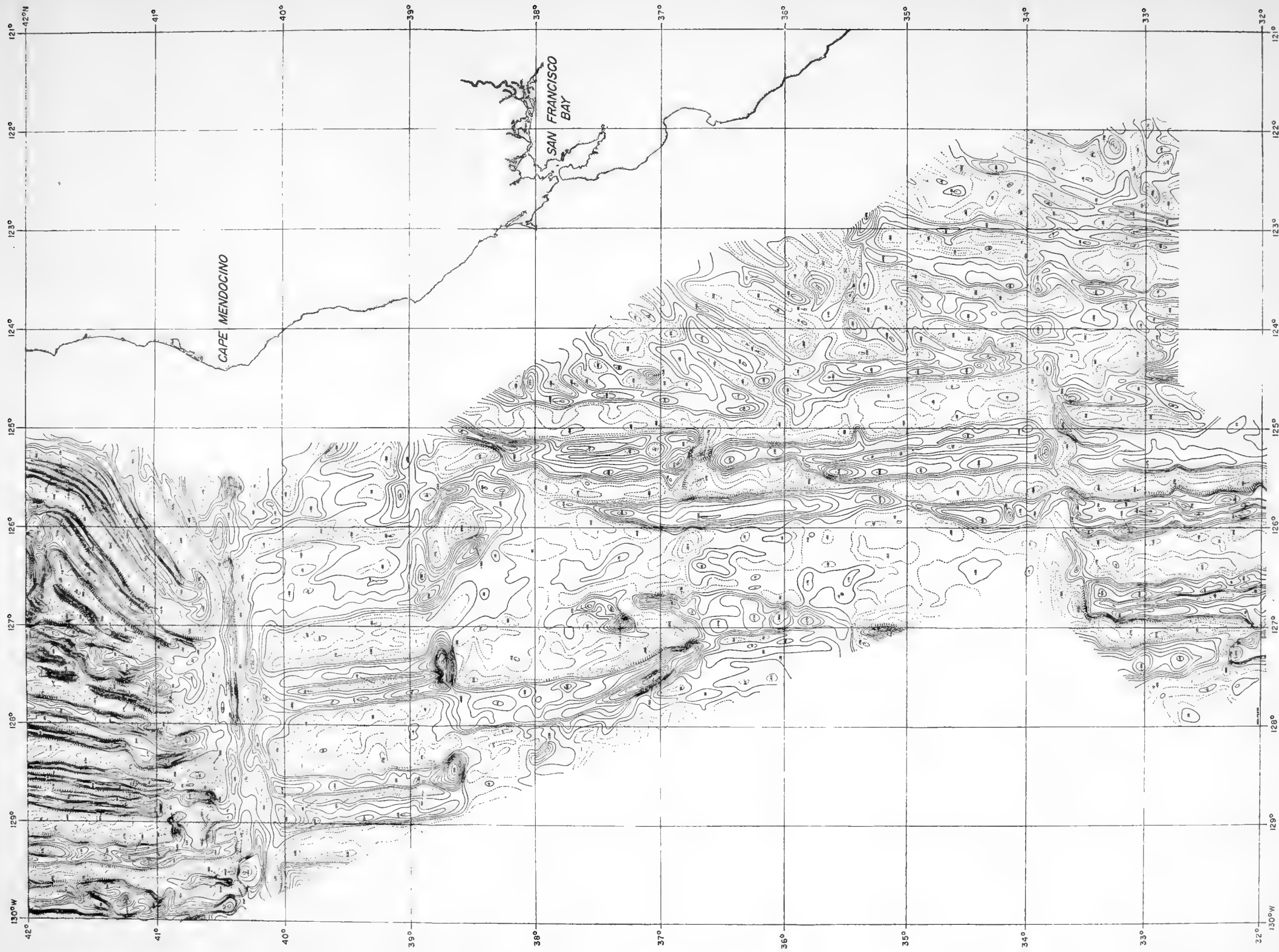
Fig. 11a. Map of the total magnetic intensity from 32°N to 42°N after removal of the regional field. The contour interval is 5 \gamma , and spot values are rounded off to the nearest 5 \gamma beyond the extreme value recorded. (From Mason and Raff, 1961.)
